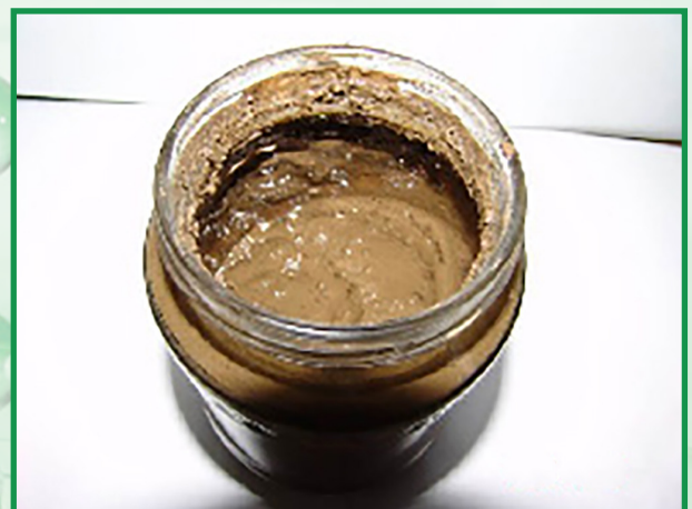
8. Oil-contaminated ground worked by Living-culture enzyme preparation 14th day
