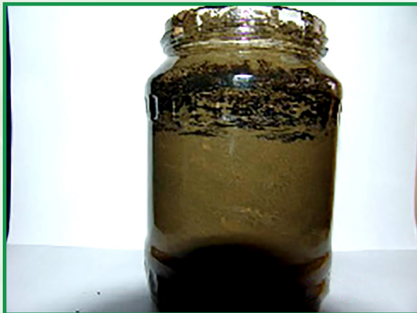
7. Oil-contaminated ground worked by Living-culture enzyme preparation 10th day
