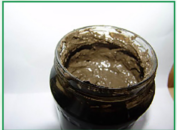
7. Oil-contaminated ground worked by Living-culture enzyme preparation 10th day
